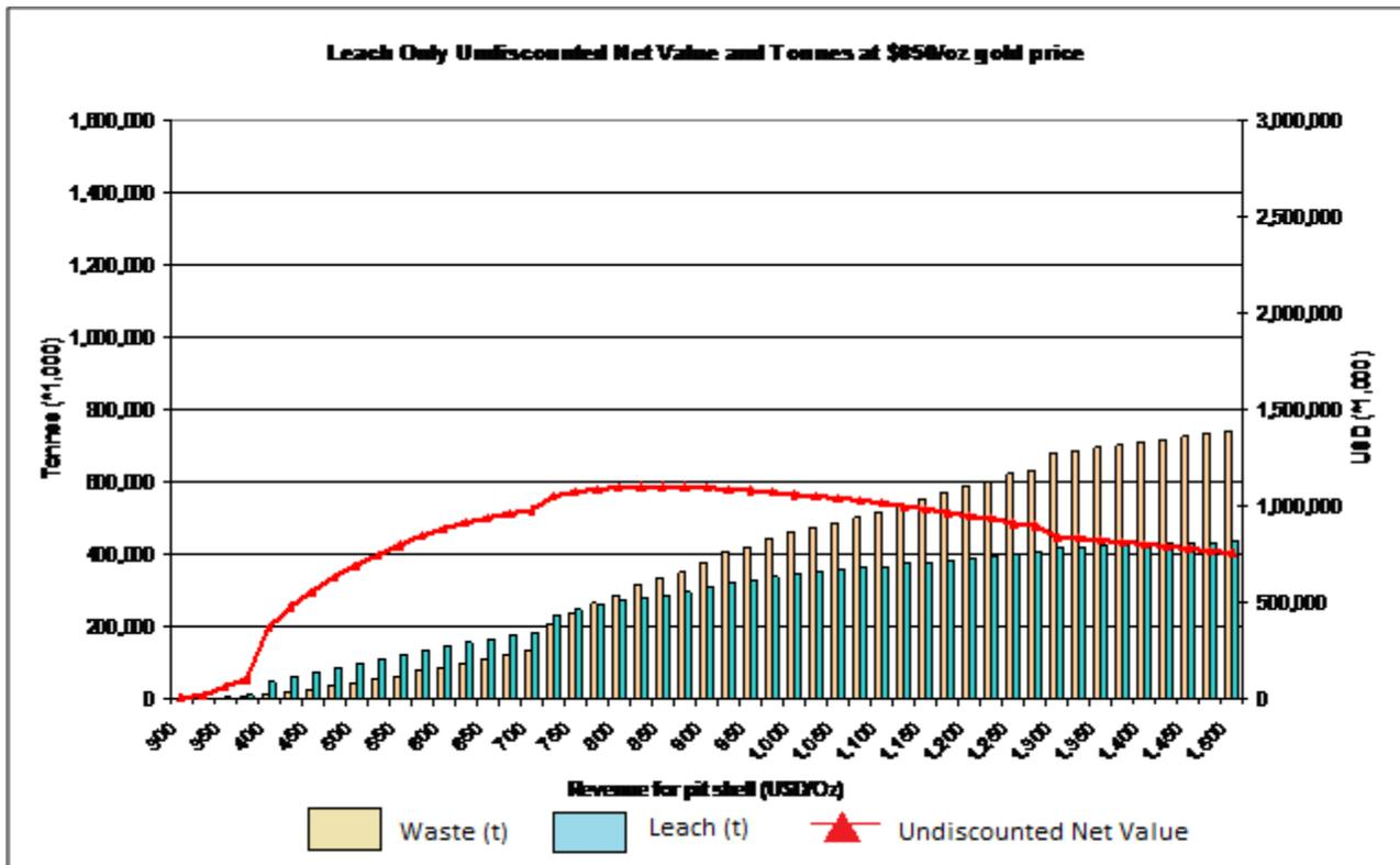
**Figure 18.1.** Leach tonnes, waste tonnes and undiscounted net value for heap leach only pit shells versus gold price.
