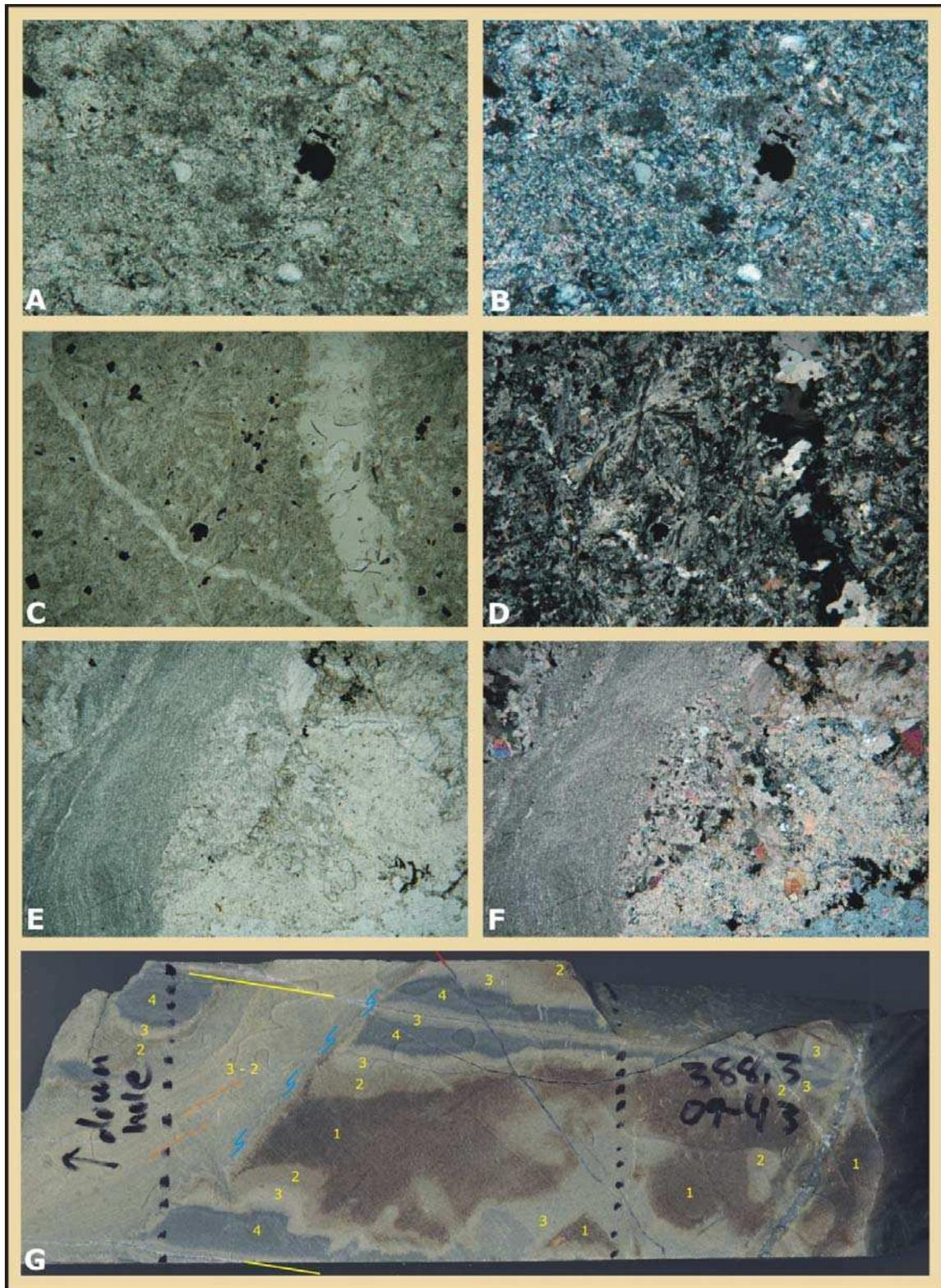
**Figure 9.4.** Photomicrographs of characteristic alteration among rocks at Money Knob - plain light on the left; crossed polarized light on the right. **A and B)** Sericite and carbonate replace a silty phyllite
