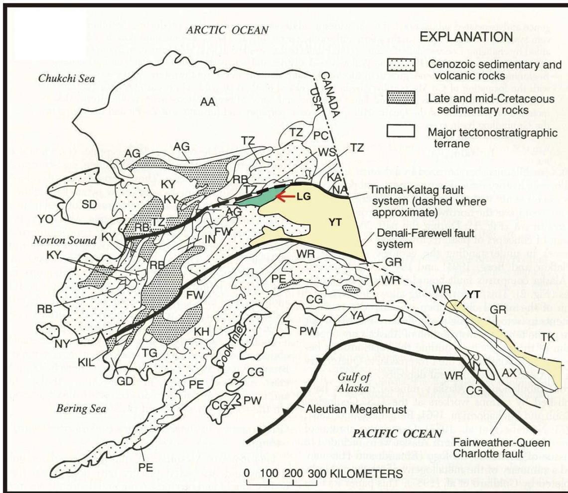
**Figure 7.1.** Terrane map of Alaska showing the location of the Livengood Terrane (LG; red arrow). The heavy black line north of the Livengood Terrane is the Tintina Fault. The heavy black line to the south of the Livengood and Yukon – Tanana Terrane (YT) is the Denali Fault. The Tintina Gold Belt lies between these two faults. After Goldfarb, 1997.
