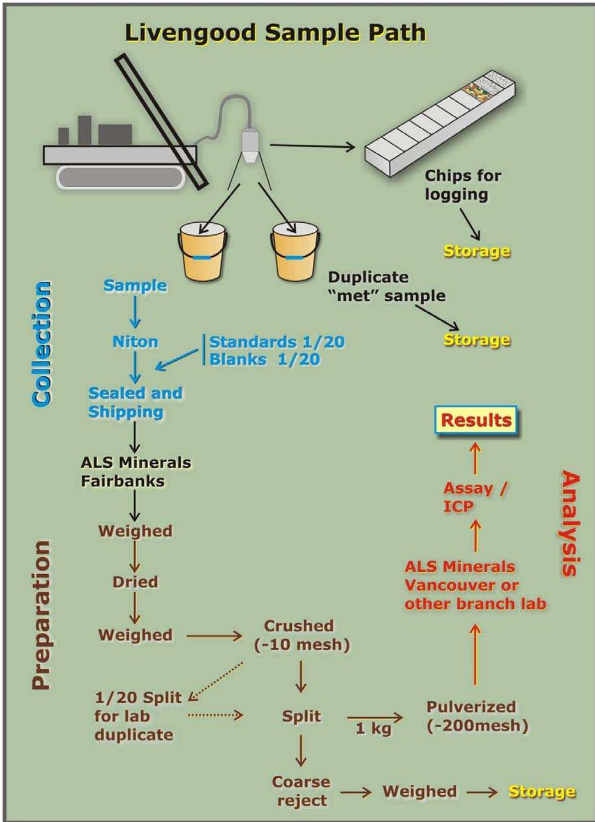
**Figure 13.1.** This diagram shows the flow path and steps involved for RC samples from the drill rig to analytical results.
