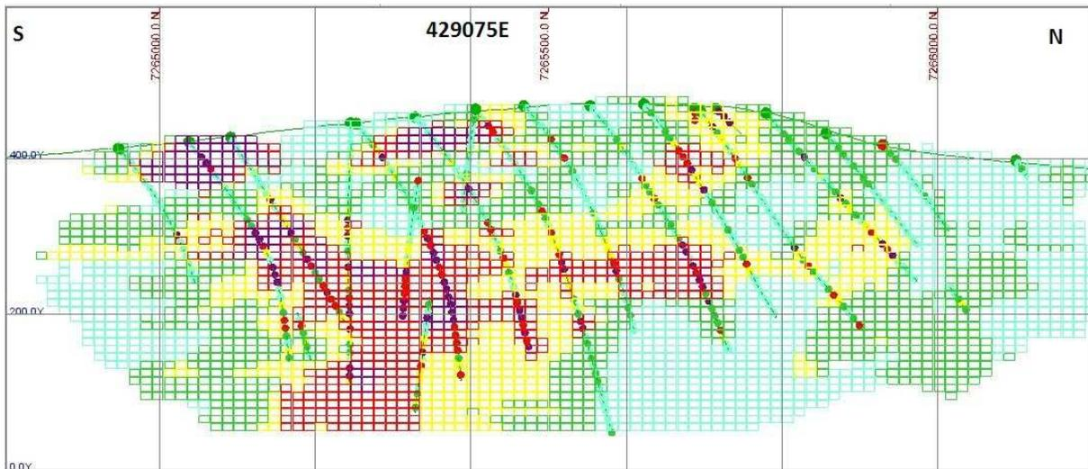
**Figure 20.4.** Block model for section 429075 E. Grid squares are 200m.
