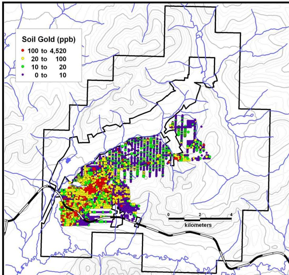
**Figure 9.1.** Plot of soil samples. Color coding shows relative gold content with red indicating gold  $\geq 0.100$  g/t Au.
