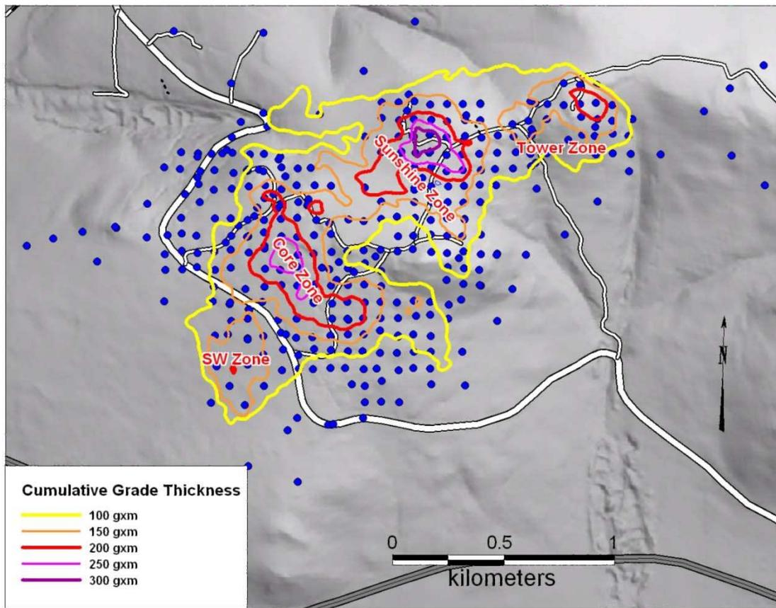
**Figure 9.2.** Cumulative gold grade thickness (March 2010) for the block model of the Money Knob deposit showing the four main zones within the deposit.
