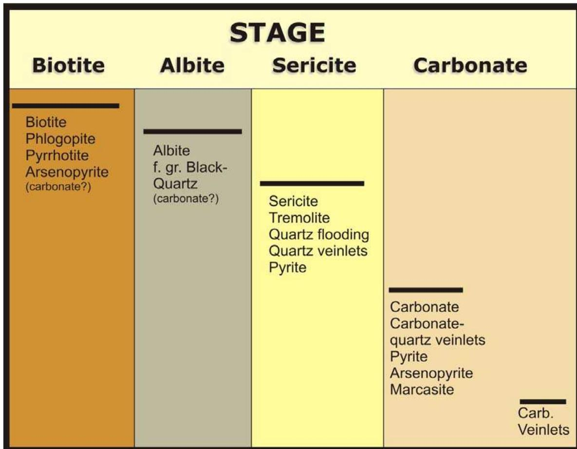
**Figure 9.5.** Interpreted paragenetic sequence of key alteration and mineralization stages. Gold occurs with arsenopyrite and may have been introduced during all stages or dominantly during a particular stage(s).
