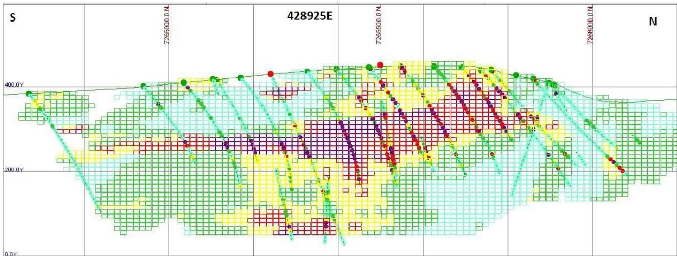
**Figure 20.3.** Block model for section 428925 E. Grid squares are 200m.
