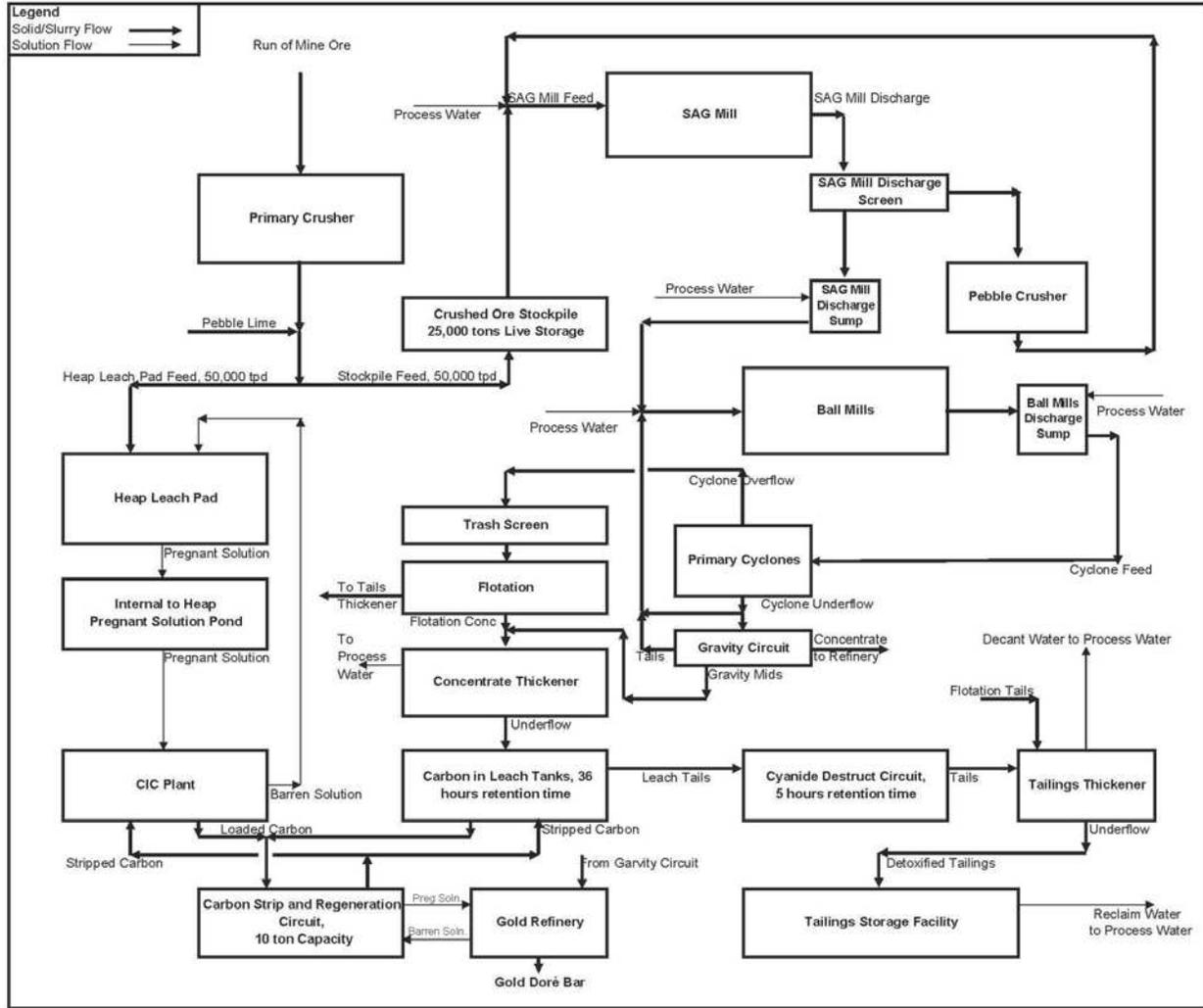
**Figure 16.3** Alternate Livengood process block flow diagram showing both Heap Leach and Mill utilizing Gravity/Flotation/Concentrate CIL process streams.
