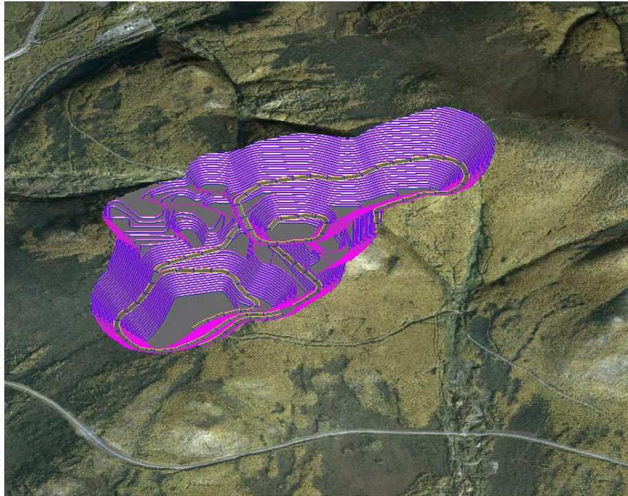
**Figure 18.5.** Mill and Heap Leach Pit Design shown in a geo-referenced photograph of the Money Knob area.
