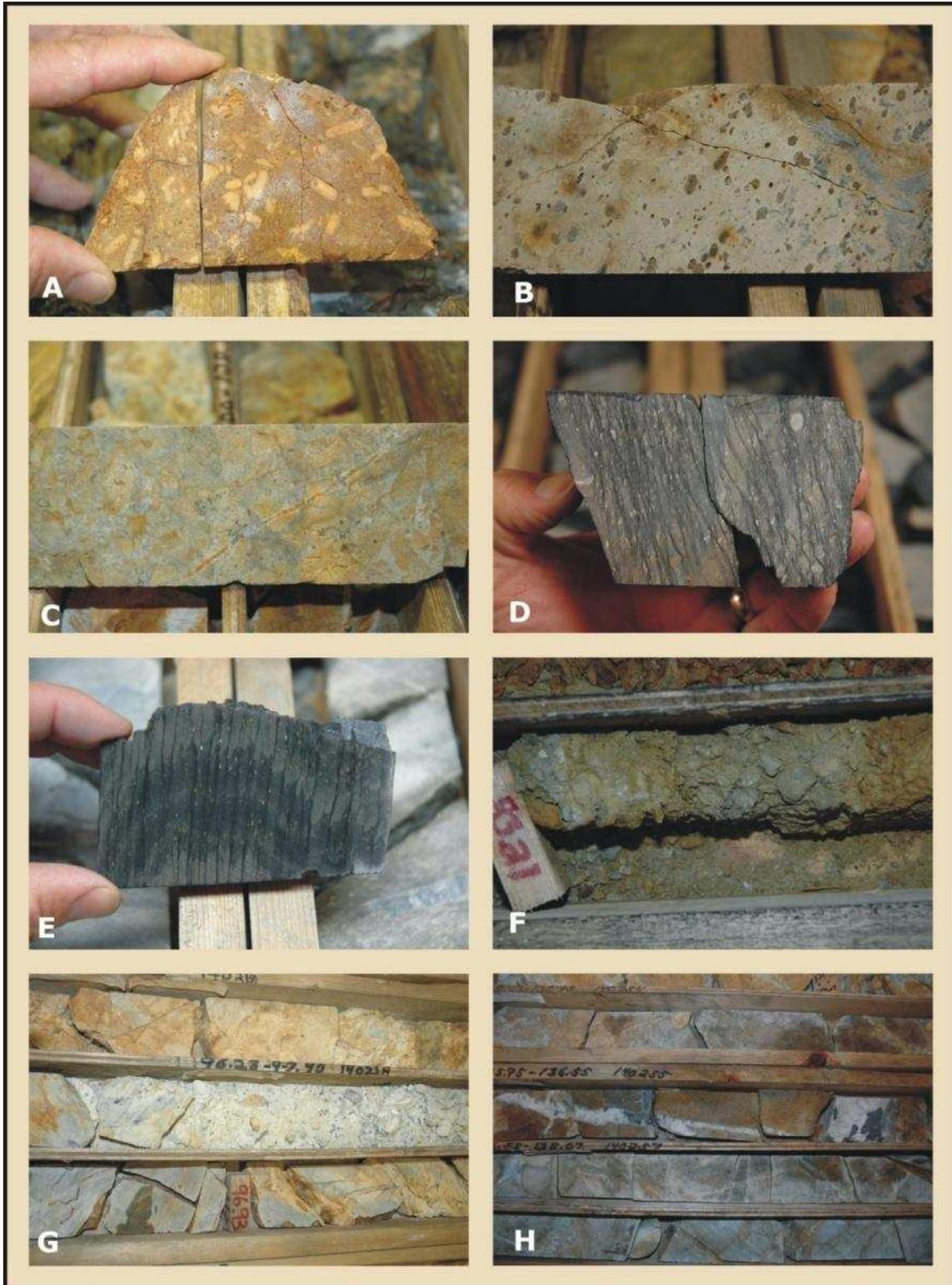
**Figure 7.6.** Photographs of key rock types and mineralization features. **A)** porphyry dike; MK07-18, 41.2 m; 1.01 g/t Au. **B)** amygdaloidal volcanic, presumably a flow, with possible Na alteration; MK07-18, 152-189. **C)** silicified volcanic breccia; MK07-18. **D)** argillite with more silty band and coral hash;
