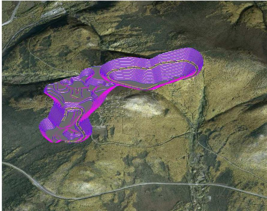
**Figure 18.2.** Heap leach only pit design shown in a geo-referenced photograph of the Money Knob area.
