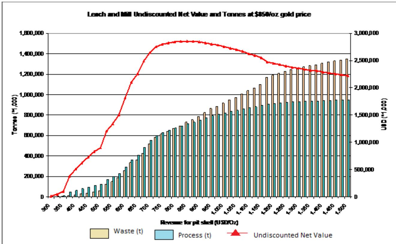
**Figure 18.4. Process feed tonnes, waste tonnes and undiscounted net value for Heap Leach and Mill pit shells versus gold price.**
