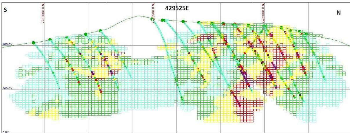
**Figure 20.5.** Block model for section 429525 E. Grid squares are 200m.
