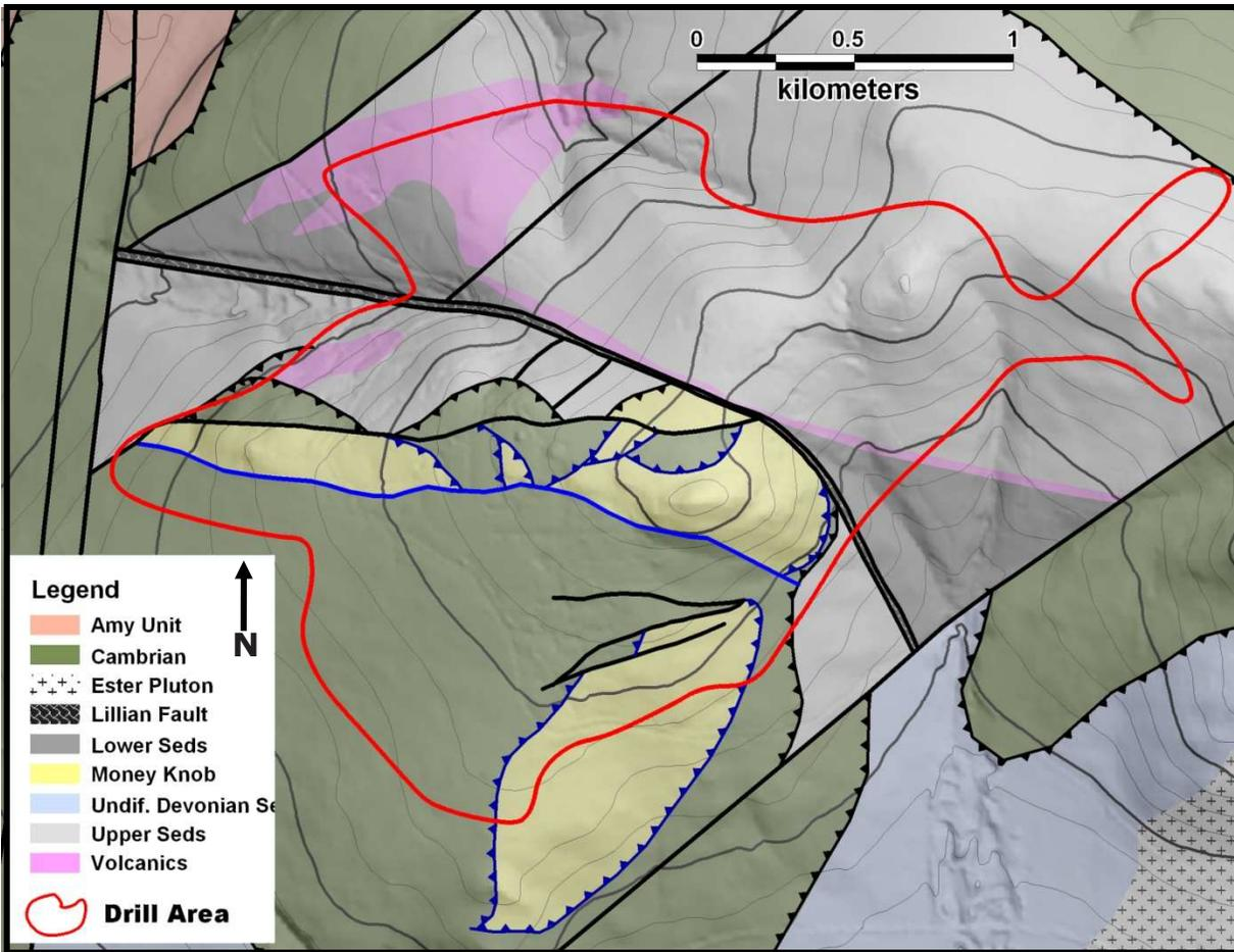
**Figure 7.4.** Generalized geologic map of the Money Knob area based on geologic work by ITH.
