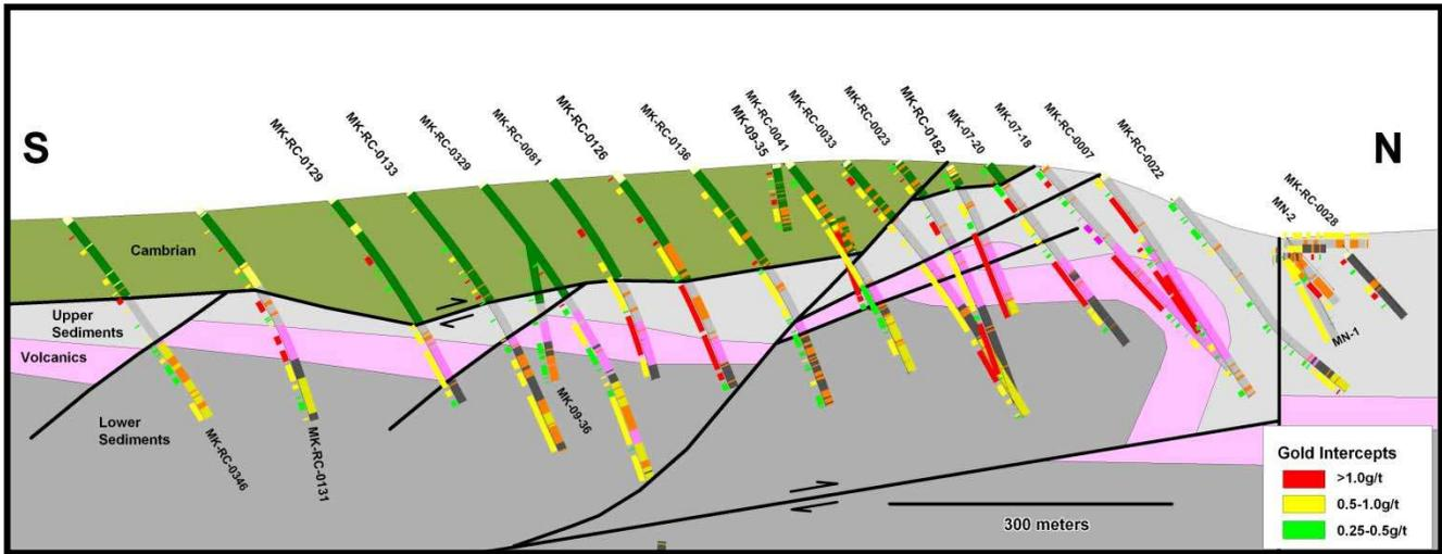
Figure 7.9. N-S Section 428850 illustrates the southerly dip of high grade zone (red) along the general stratigraphic pattern.
