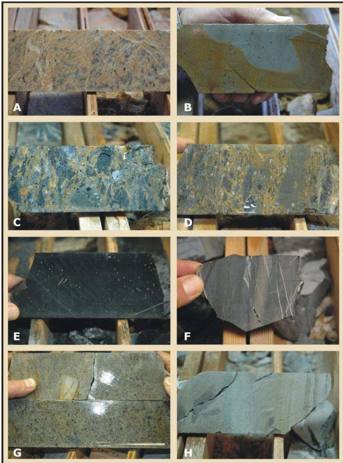
**Figure 7.5.** Photographs of key rock types at Livengood. **A)** ultramafic rock with carbonate alteration (yellow-brown); MK7-20, 13.5m; **B)** siltstone with carbonate and pyrite knots. Brown color is oxidation front. MK 07-18, 8.5m **C)** sedimentary conglomerate; at least some clasts appear to be rip-up clasts of
