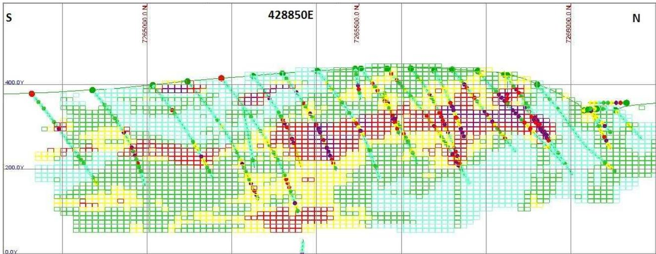
**Figure 20.2.** Block model for section 428850 E. Grid squares are 200m.
