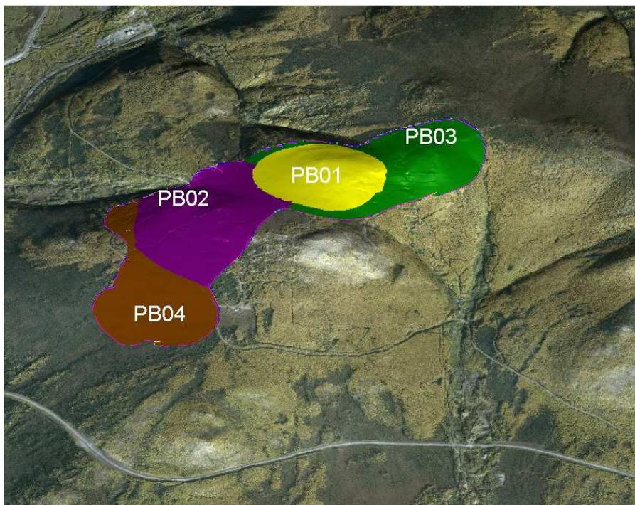
**Figure 18.3.** Pushbacks used for heap leach only production scheduling.
