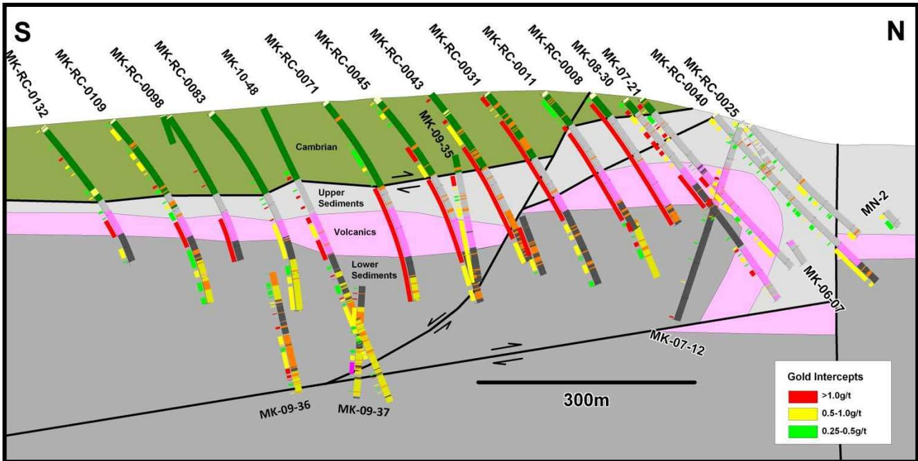
Figure 7.10. N-S Section 428925 illustrates the general southerly dip of mineralization and how it lies along the stratigraphic and structural grain.
