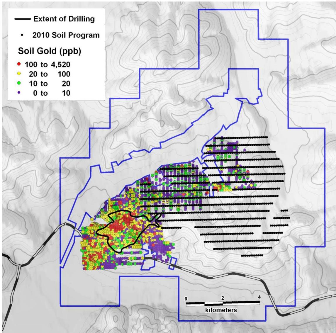
**Figure 11.1.** Distribution of drilling in the Money Knob area with respect to anomalous soil samples. The majority of the soil geochemical target remains untested. An expanded soil sampling program is proposed for 2010.
