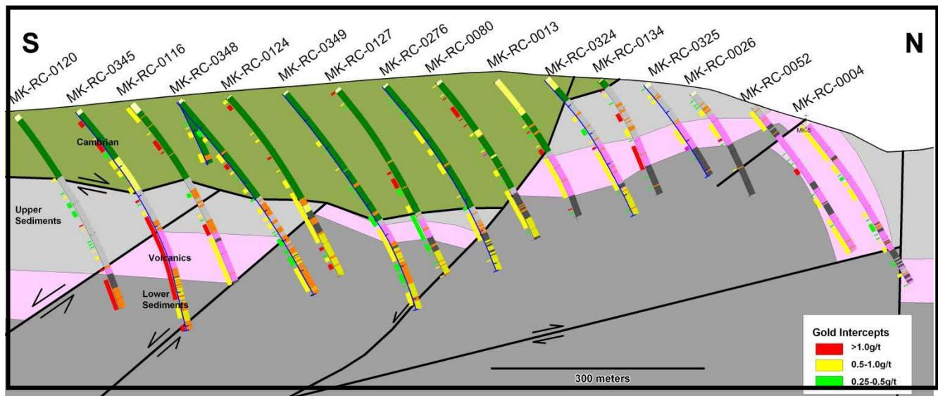
**Figure 7.8.** N-S Section 428625 E illustrates the complexities of thrust and normal fault interpretation and shows the southerly dip of high grade zones (red).
