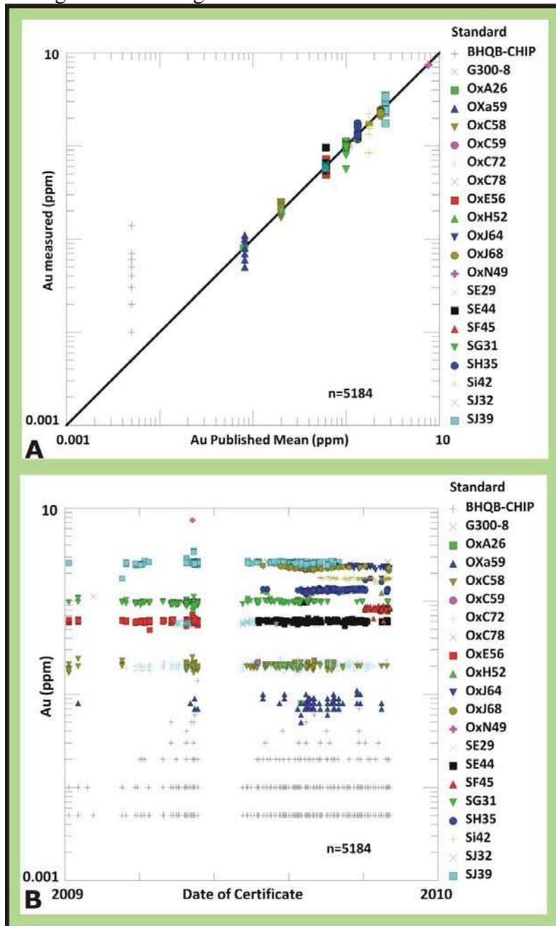
Figure 13-3 X-Y scattergrams for 2009 showing the stated value of standards vs. the measured value by the lab
