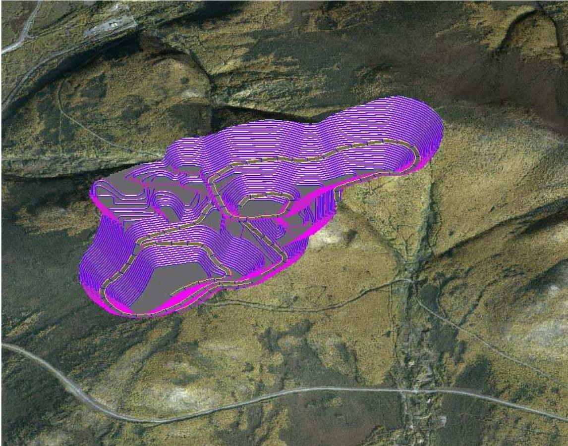
**Figure 18-5 Mill and Heap Leach Pit Design shown in a geo-referenced photograph of the Money Knob Deposit Location.**
