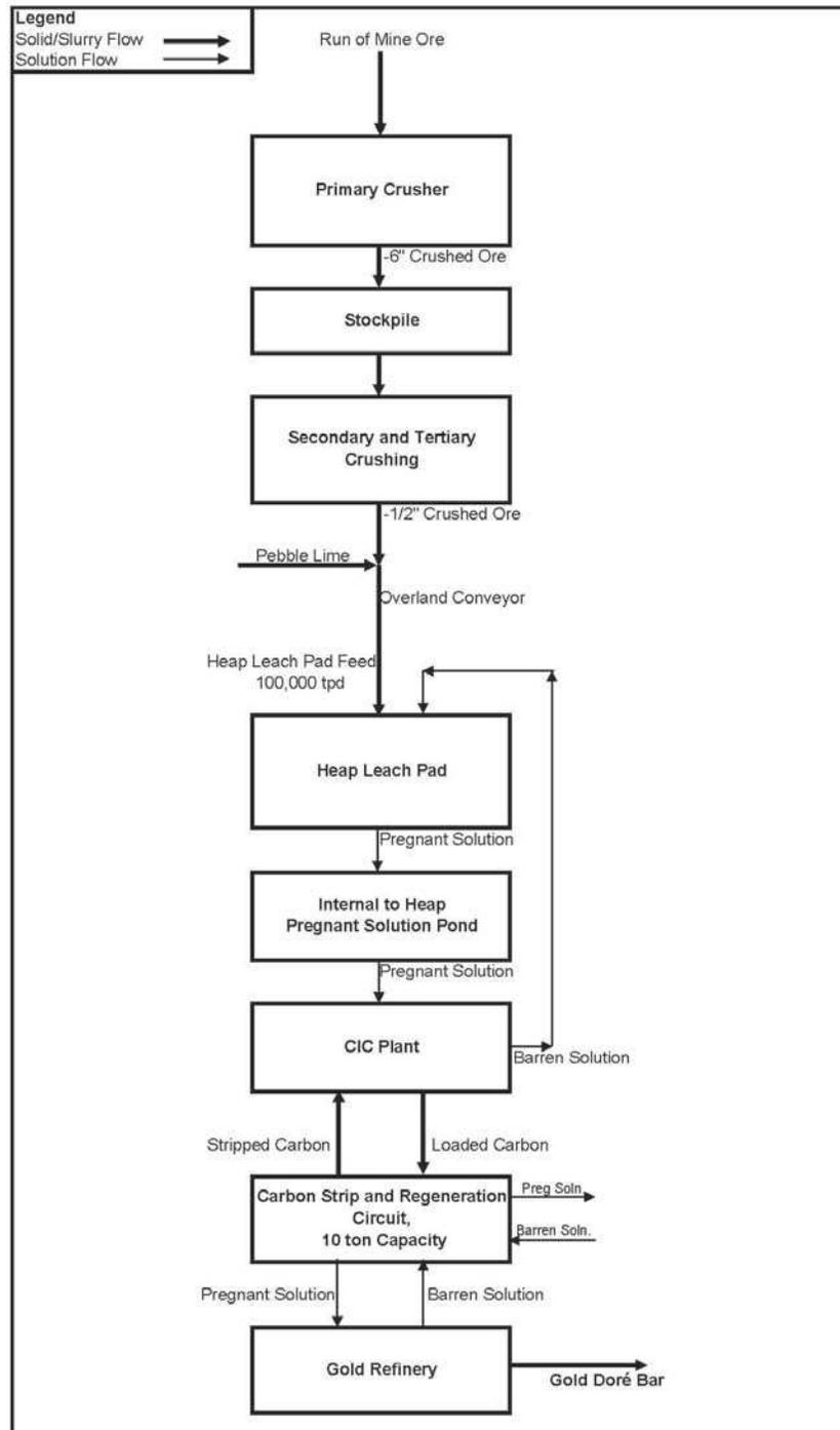
Figure 16-1 Proposed Livengood process block flow diagram showing heap leach process streams.
