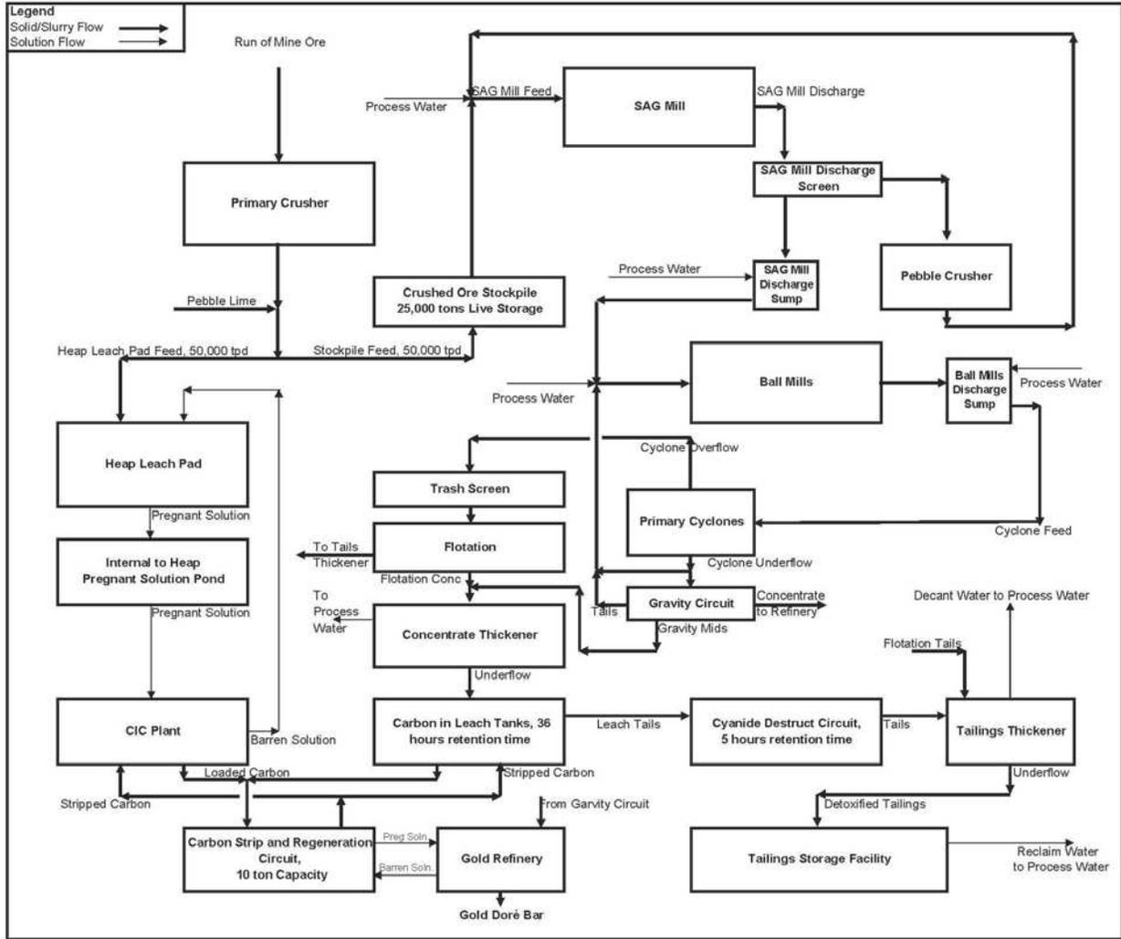
Figure 16-2 Alternate Livengood process block flow diagram showing both Heap Leach and Mill utilizing Gravity/Flotation/Concentrate CIL process streams.
