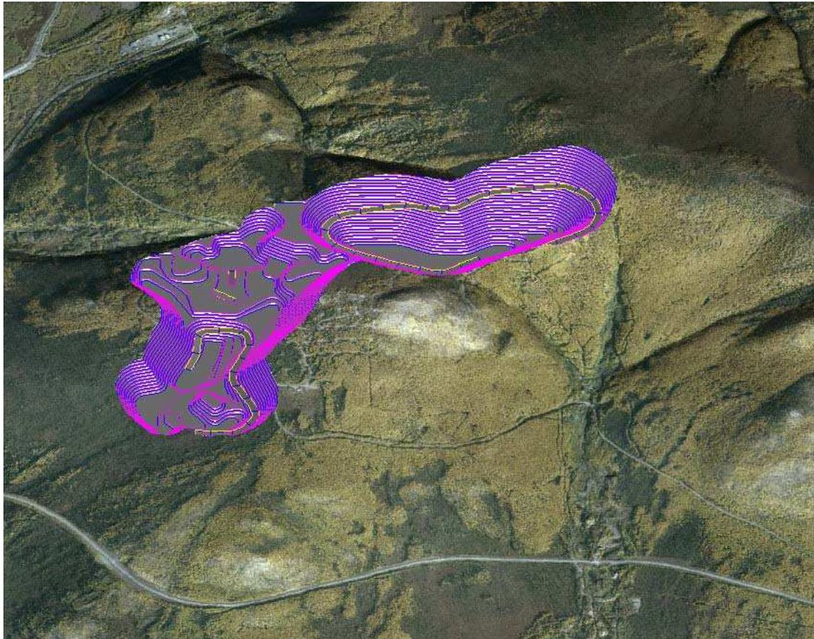
Figure 18-2 Heap Leach Only Pit Design shown in a geo-referenced perspective view of the Money Knob Deposit Location. North is toward the top of the view.
