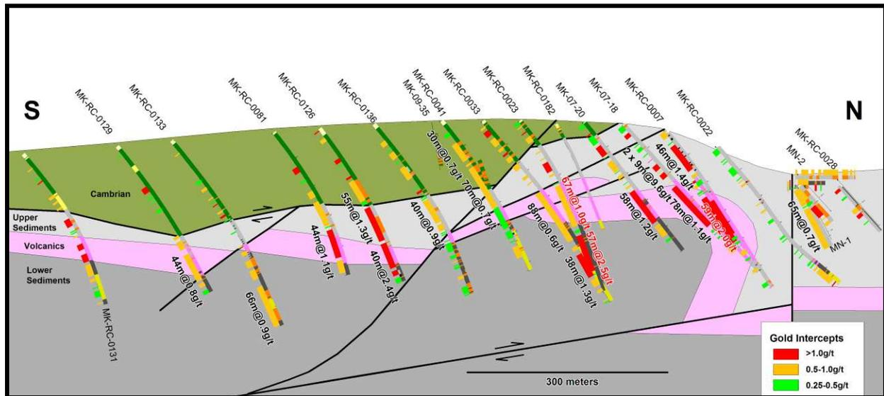
Figure 7.9. N-S Section 428850 illustrates the southerly dip of high grade zone (red) along the general stratigraphic pattern.
