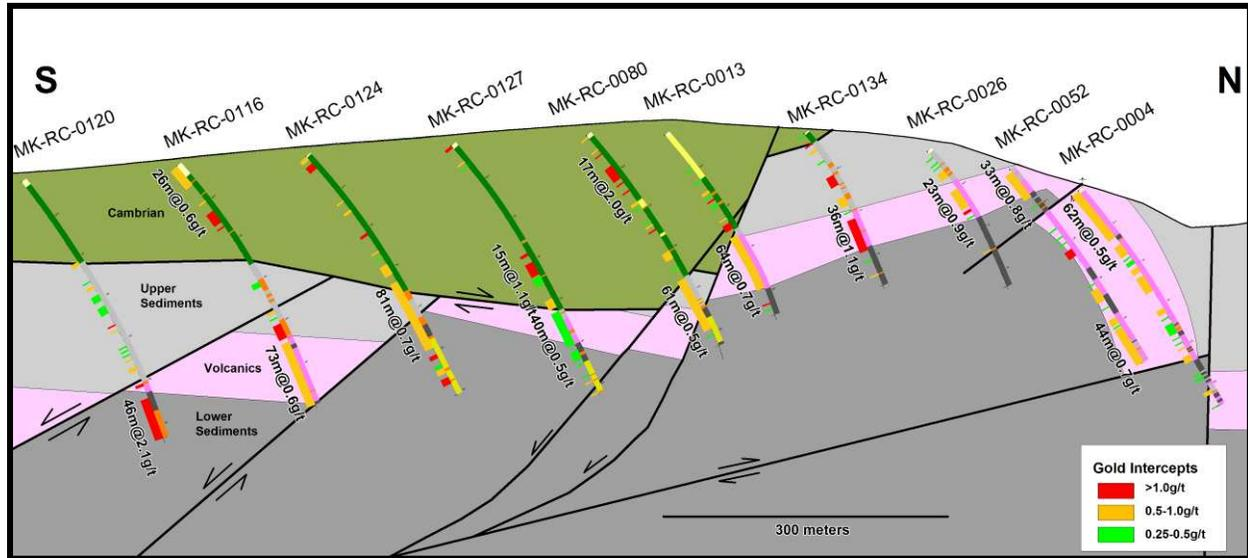
Figure 7.8. N-S Section 428625 E illustrates the complexities of thrust and normal fault interpretation and shows the southerly dip of high grade zones (red).
