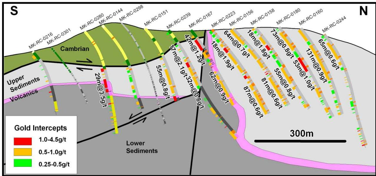
**Figure 7.12.** N-S Section 429675 illustrates the pattern of mineralization reflecting structural and stratigraphic controls.
