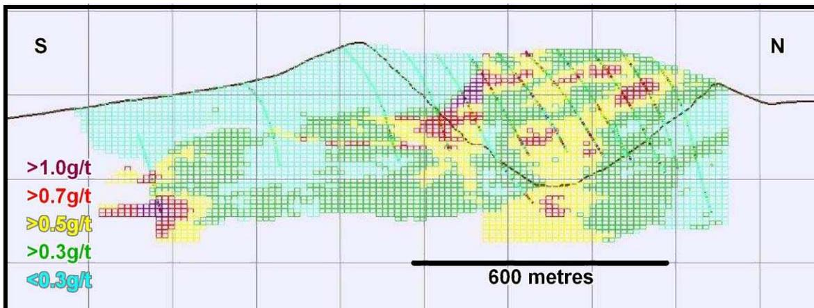
Figure 19.3. Block model for section 429675 E.
