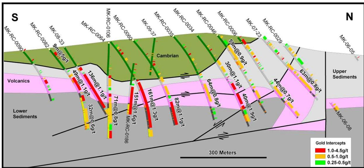
**Figure 7.11.** N-S Section 429075 illustrates the pattern of mineralization reflecting structural and stratigraphic controls.
