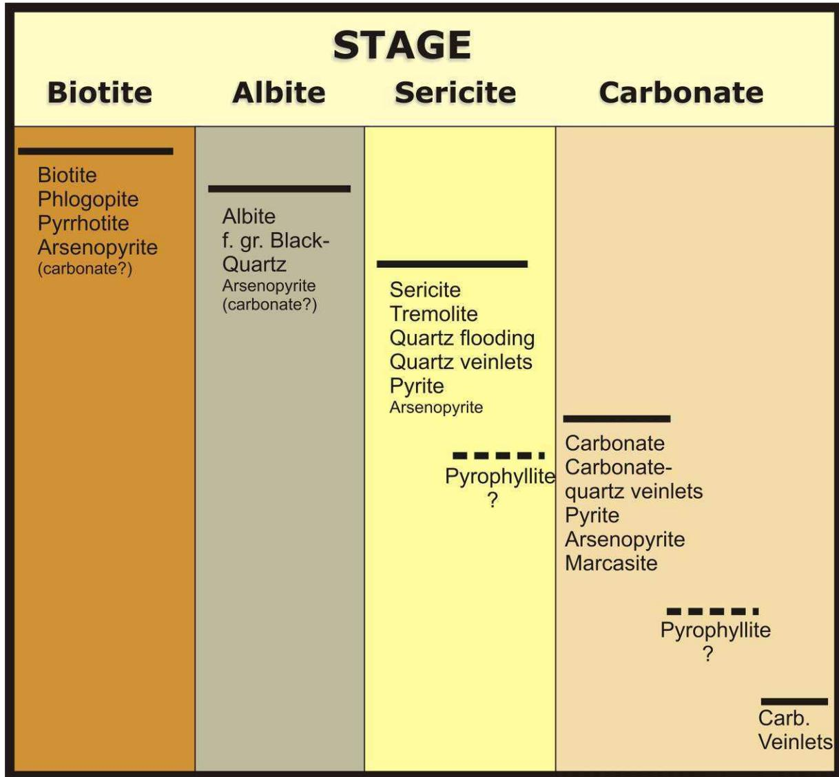
**Figure 9.4** Interpreted paragenetic sequence of key alteration and mineralization stages. Gold occurs with arsenopyrite and may have been introduced during all stages or dominantly during a particular stage(s). It is not clear where smectite-illite alteration might fit into this sequence.
