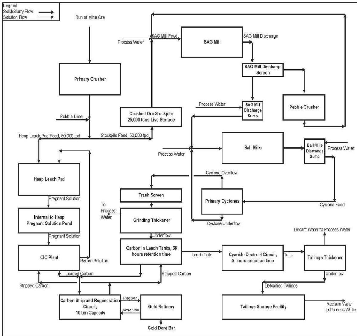
Figure 16.3 Alternate Livengood process block flow diagram showing both heap leach and mill / cil process streams
