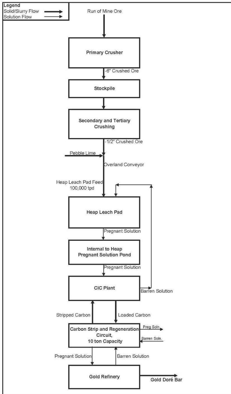
**Figure 16.2** Proposed Livengood process block flow diagram showing heap leach process streams.
