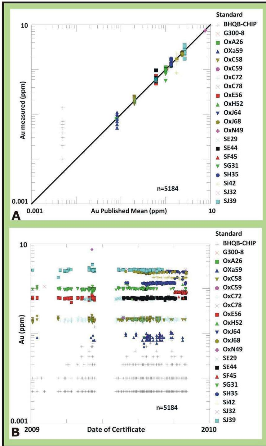
**Figure 13.2.** X-Y scattergrams for 2009 showing the stated value of standards vs. the measured value by the lab. **A)** values are plotted according to measured value vs. stated values of a standard placed in the sample stream. **B)** values plotted as a function of time to check for drift in results over time. The horizontal nature of the points for each value indicates that drift is minimal to non-existent.
