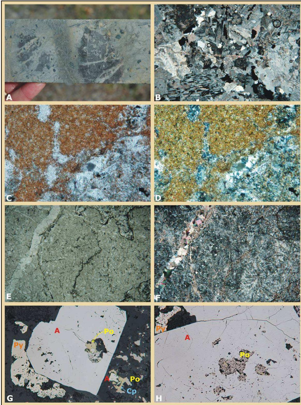
**Figure 9.2.** Photomicrographs of characteristic alteration among rocks at Money Knob. A) View of core showing relict patches of secondary biotite (dark color) cut by and overprinted by albite and
