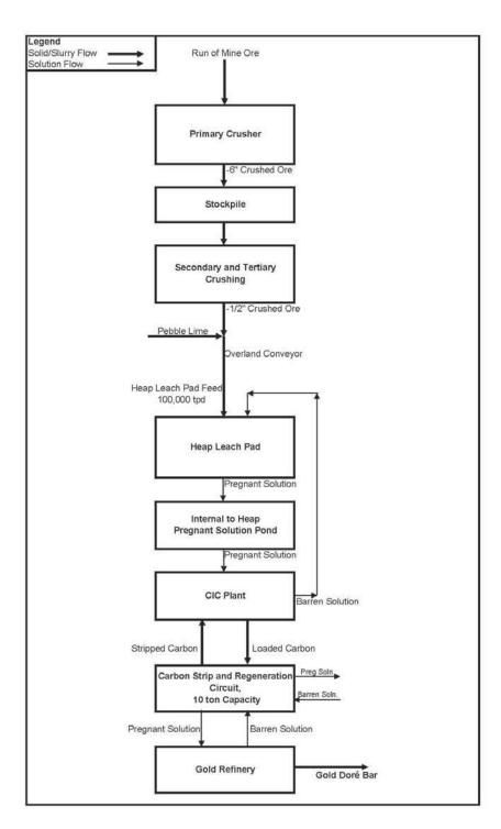
**Figure 16.2.** Proposed Livengood process block flow diagram showing heap leach process streams.
