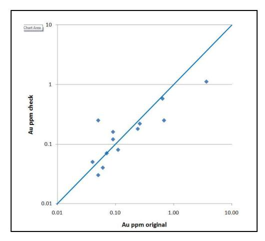
**Figure 14.2.** X-Y scatter plot of original and check samples for June 2009 RC drilling. The correlation line shows a slope of 1. Samples with identical results will plot on the line. Deviation of results from the line is interpreted to be the result of normal variation and nugget effect.
