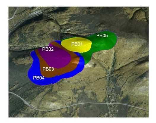
Figure 18.6. Pushback forming the basis of the combined heap leach and mill production schedules.
