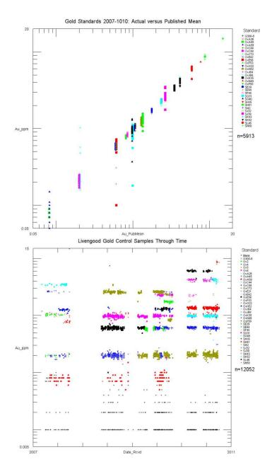
**Figure 13.3.** X-Y scattergrams for 2007 - 2010 showing the stated value of standards vs. the measured value by the lab: **Top)** values are plotted according to measured value vs. stated values of a standard placed in the sample stream. **Bottom)** values plotted as a function of time to check for drift in results over time. The horizontal nature of the points for each value indicates that drift is minimal.
