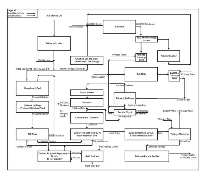
**Figure 16.3** Alternate Livengood process block flow diagram showing both Heap Leach and Mill utilizing Gravity/Flotation/Concentrate CIL process streams.
