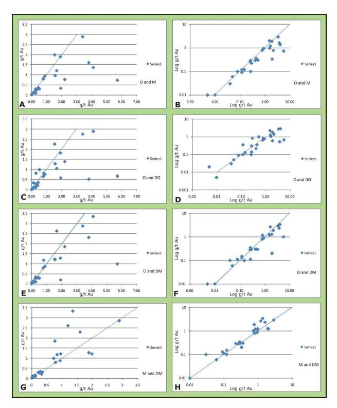
**Figure 14.1.** X-Y scatter plots of 2008 and early 2009 original and duplicate sample data for check samples collected by Dr. Klipfel as part of data validation procedures. The diagrams on the left are plotted with numeric scales. The diagrams on the right are plotted with log-log scales. The scatter increases with grade on diagrams with numeric scales while the envelope of points remains approximately parallel to the "unity" line. This is consistent with data following lognormal abundance
