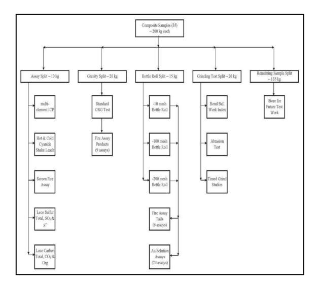
**Figure 16.1.** Flow chart and breakdown of Livengood composite sample test work.
