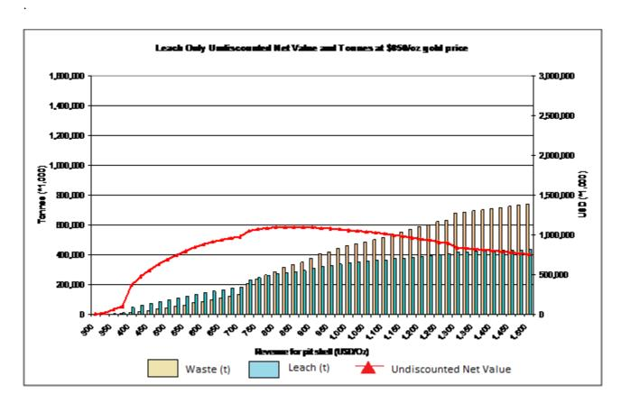
**Figure 18.1.** Leach tonnes, waste tonnes and undiscounted net value for heap leach only pit shells versus gold price.
