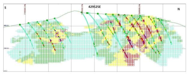
**Figure 20.5.** Block model for section 429525 E. Grid squares are 200m.
