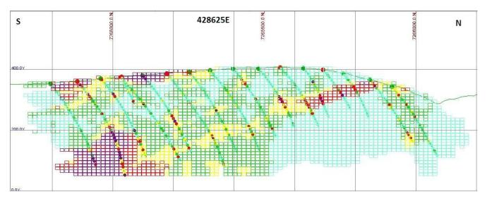
Figure 20.1. Block model for section 428625 E. Grid squares are 200m.
