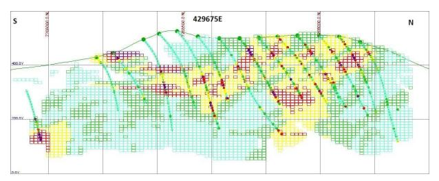
Figure 20.6. Block model for section 429675 E. Grid squares are 200m.
