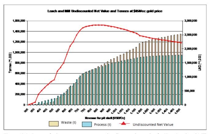
**Figure 18.4. Process** feed tonnes, waste tonnes and undiscounted net value for Heap Leach and Mill pit shells versus gold price.
