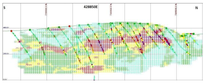
Figure 20.2. Block model for section 428850 E. Grid squares are 200m.
