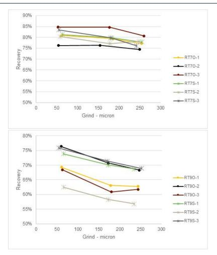
Figure 10-39: Overall gold recovery according to grind size (2021 PFS – Phase 11)
