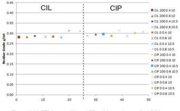
Figure 10-27: RT9 Average CIL and CIP residue grades at a  $P_{80}$  of 113  $\mu m$   $(2021\mbox{ PFS}-\mbox{Phase }9a)$
