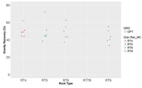
Figure 10-6: Gold gravity concentration grind-recovery relationships for RT4, RT5, RT6 and RT9 (FS)
