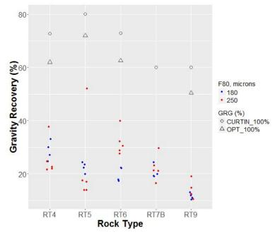
Figure 10-14: 2017 PFS (Phase 9) gravity recovery for all tock types (GRG presented as the 3<sup>rd</sup> stage of GRG)
