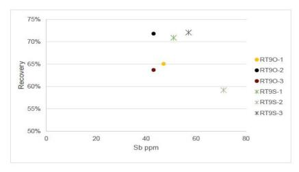
Figure 10-38: Overall gold recovery according to location inside or outside the 100 ppm Sb shell  $(2021\ \text{PFS}-\text{Phase 11})$
