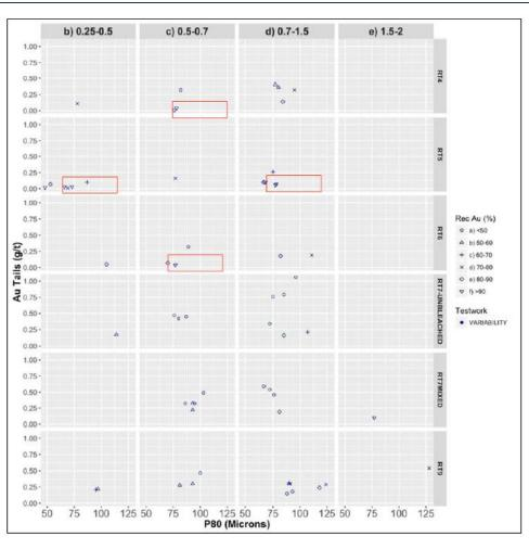
Figure 10-12: Gold in Residues from CIL testwork vs  $\mathsf{P}_{80}$  for each rock type (FS)
