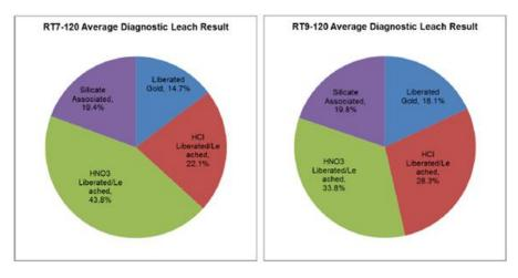
Figure 10-34: Diagnostic leach result distribution (2021 PFS – Phase 9b)
