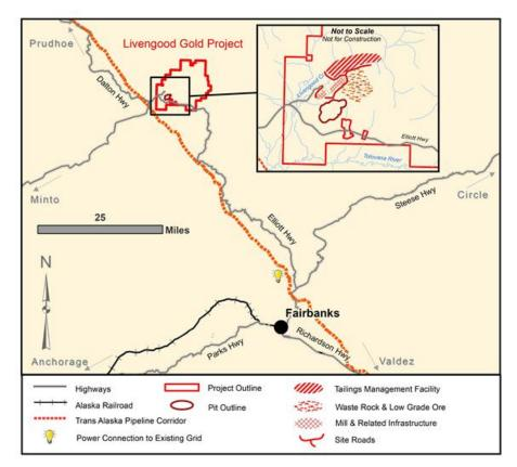
Figure 15-1: Livengood property – conceptual infrastructure arrangement drawing
