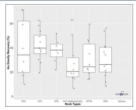
Figure 10-11: Gold gravity recovery box plots (FS)
