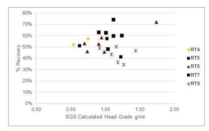
Figure 10-37: Gravity recovery vs calculated head by rock type (2021 PFS – Phase 11)
