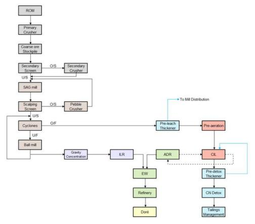
Figure 14-1: Conceptual process block flow diagram
