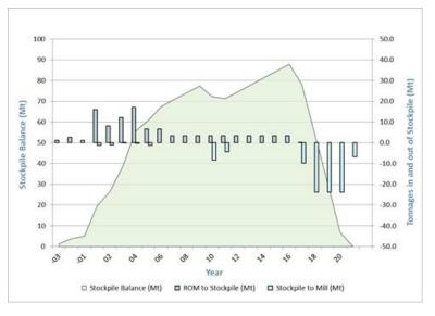
Figure 13-11: Low grade ore stockpile balance
