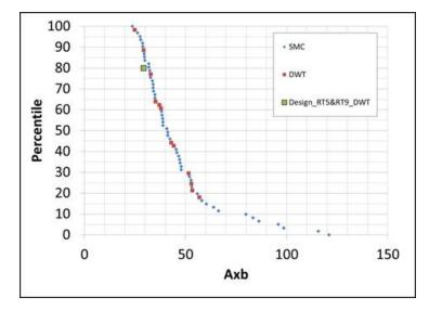
Figure 10-3: Cumulative A × b (DWT + SMC) results for the Livengood Gold Project
