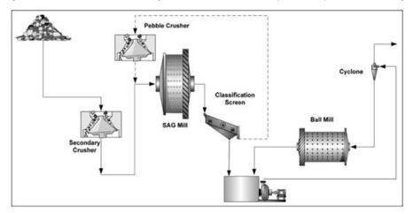
Figure 10-5: SABC with pre-crushing (secondary crusher) circuit configuration
