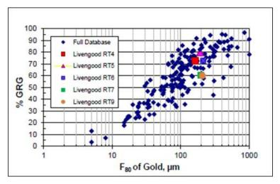
Figure 10-17: Livengood GRG results vs FLS/Curtin database (source Curtin report) (2017 PFS)
